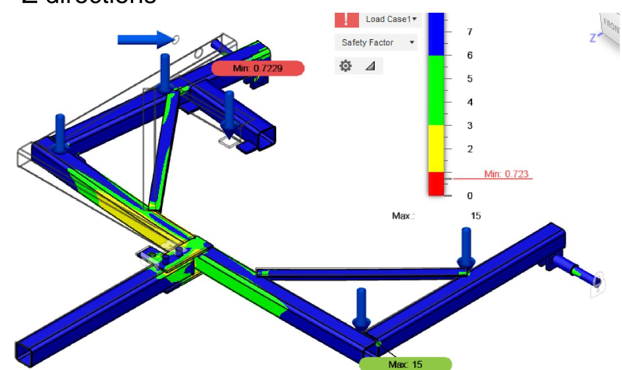
This was a static analysis of the worst case scenario of an impact on the wheel from a collision. The weakest point is at the spindle. Since the frame is strong enough to handle this worst case scenario, it will be strong enough to handle day-to-day use.
